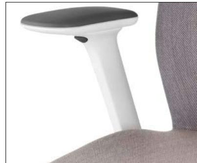
The height of the **standard 1D-armrests** is adjustable by 100 mm (3 $\frac{7}{8}$ ") at the touch of a button. The depth of the armrest pads on 3D armrests can optionally be extended by 50 mm (2") and the width by 25 mm (1"), 4D armrests can also rotate inwards and outwards by 25°.
